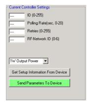
Retries: In Peer-to-Peer mode, this parameter determines the number of consecutive failed polling attempts before a communications failure occurs. It is not recommended to set the number of retries higher than 10 attempts. Large numbers may cause an unnecessary delay in communications failure response time; a low number may cause the system to prematurely fail. This parameter has no affect in Modbus mode.
